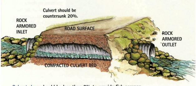
Culvert slope should be less than 2% to provide fish passage.
