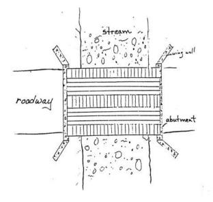
Wingwalls should be of sufficient height and length to prevent anv roadfill from entering the stream. Acceptable wingwall materials are steel, treated concrete, wood or rock riprap.
