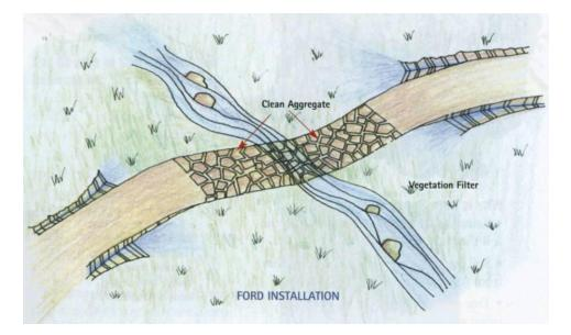
Gently sloping, stable streambank approaches are preferred. Approaches should be rocked to minimize erosion when driving in and out of the ford. Where practical, approaches should be at right angles to the stream. Approaches should dip into and out of the stream, creating a concave shape that ensures the stream cannot be diverted out of its natural channel and down the road.
