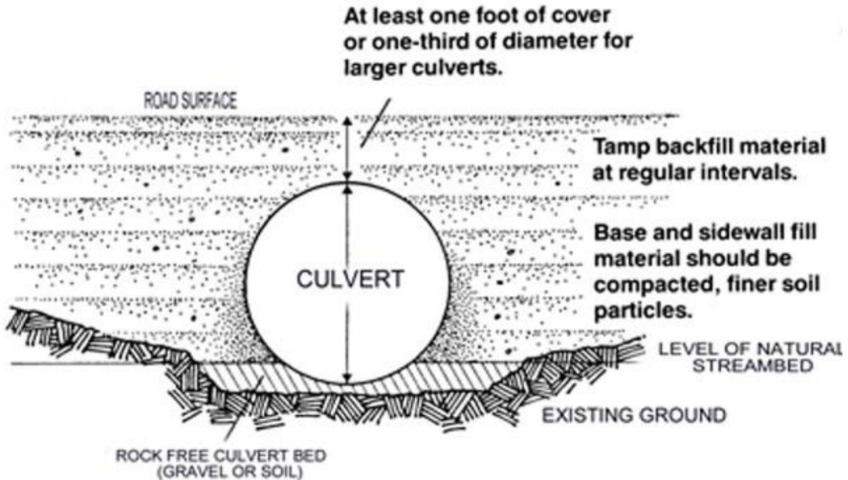
Tamping fill material in layers (lifts) throughout the entire backfill process is important. The base and sidewall material should be compacted first. This reduces seepage into the fill.
