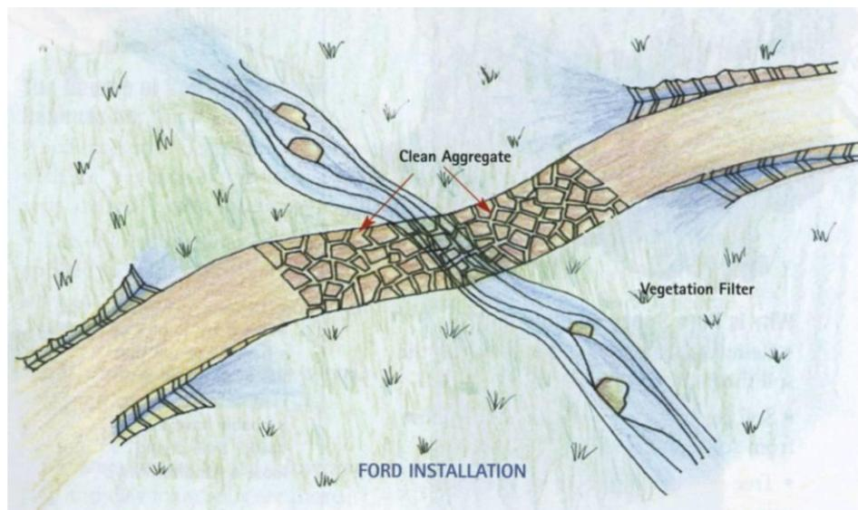
Gently sloping, stable streambank approaches are preferred. Approaches should be rocked to minimize erosion when driving in and out of the ford. Where practical, approaches should be at right angles to the stream. Approaches should dip into and out of the stream, creating a concave shape that ensures the stream cannot be diverted out of its natural channel and down the road.
