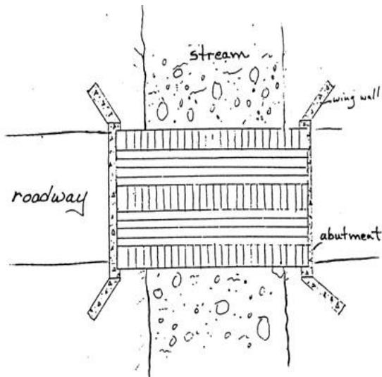
Wingwalls should be of sufficient height and length to prevent any roadfill from entering the stream. Acceptable wingwall materials are concrete, steel, treated wood or rock riprap.
