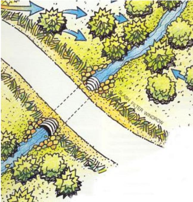
Install stream crossing at right angles to the channel whenever possible.
